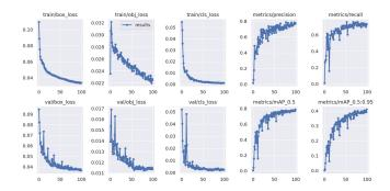
Figure 6: The model's accuracy and recall gradually increase and converge over time. Around the 25th epoch, the growth rate of both accuracy and recall starts to slow down. The mean Average Precision (mAP) exhibits a similar growth curve, eventually stabilizing at around 0.8. Overall, the model performs well on the steel surface defect dataset.
