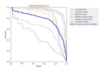
Figure 7: Among spots, pitted surface, inclusions, and scratches, individual mAPs are 0.942, 0.835, 0.830, and 0.943, surpassing the overall average. Conversely, crazing and rolled-in scale perform poorly, with mAPs of 0.447 and 0.601, impacting overall model performance.
