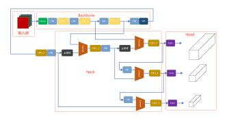
Figure 1: In the network architecture of YOLOv5, the attention module can be inserted into the last layer of the backbone network or into the Neck network to enhance feature fusion capability. In this paper, we choose to insert the attention module after the three-scale feature maps output by the Neck network. After applying the attention mechanism, the feature maps are then fed into the detection head
