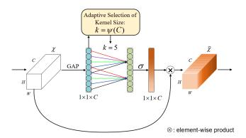
Figure 3: Efficient Channel Attention (ECA) Module
