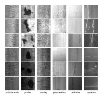
Figure 5: The presentation of some aspects of the NEU dataset reveals that there are significant visual differences among intra-class defects. For example, scratches (last column) can be horizontal, vertical, or diagonal. Similarly, inter-class defects share similarities, such as scale, crack, and pitted surface. Additionally, the grayscale variations of intra-class defect images are influenced by lighting and material changes
